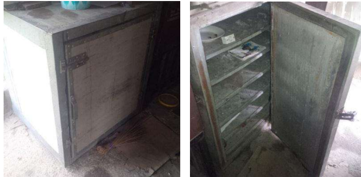
Figure 1: Local ice-making machine used as humidity chamber
